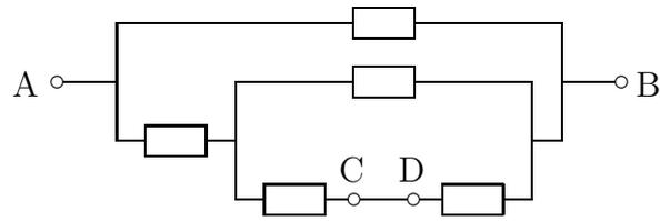
What resistance would be measured between terminals A and B? If a  $6\text{ V}$  battery with an internal resistance of  $125\ \Omega$  is connected across terminals A and B, what current flows in the wire connecting terminals C and D?
